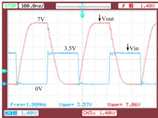
Fig. 9. (Color online) Measured input and output waveforms at 2 MHz.
