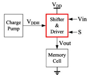
Fig. 1. (Color online) Application of level converter circuit used in the embedded nonvolatile memory.
