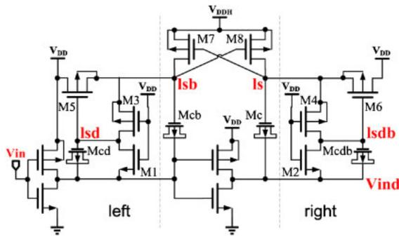
Fig. 5. (Color online) Level shifter circuit to provide the three control signals (Isd, Is, and  $V_{ind}$ ) for the driver.
