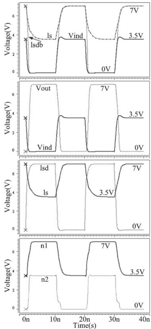
Fig. 7. Simulated waveforms of the node voltages for the driver with the output capacitance of  $0.5\text{ pF}$  at  $50\text{ MHz}$ .
