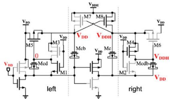
Fig. 6. (Color online) On/off state of the transistors of the level shifter when  $V_{in}$  is  $V_{DD}$ .
