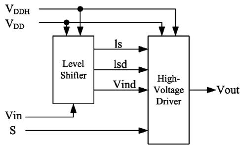
Fig. 2. Level converter consisting of two circuit blocks.
