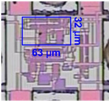
Fig. 8. (Color online) Micrograph of the proposed level converter circuit.
