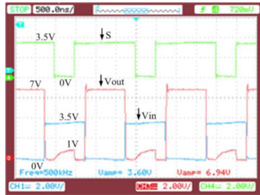
Fig. 10. (Color online) Measured waveforms with the floated output at 500 kHz.
