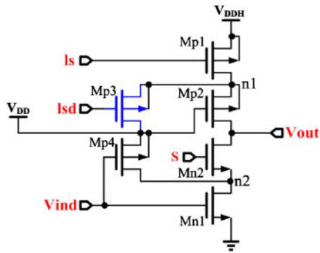
Fig. 3. (Color online) Circuits of high-voltage driver for the bit-line of memory cell.
