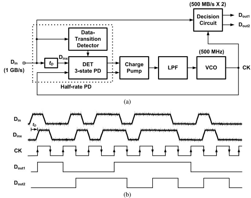
**Fig. 1** (a) Generic half-rate CDR architecture with a clock recovery circuit and a data decision circuit. (b) Corresponding waveforms.
