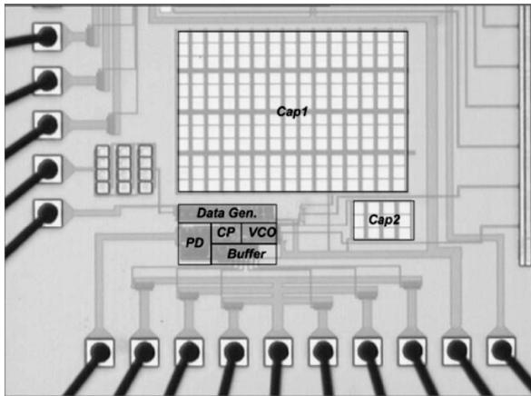
Fig. 7 Test-chip microphotograph.
