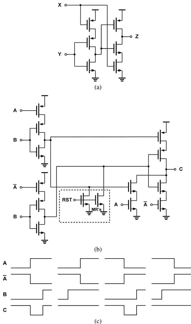
Fig. 3 (a) SET-HTR. (b) DET-HTR. (c) Timing diagram of (b).
