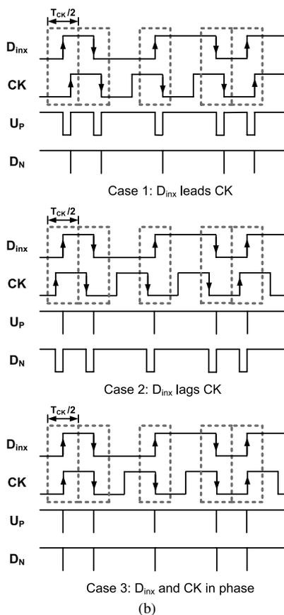
Fig. 2 Proposed half-rate phase detector for data stream. (a) Scheme. (b) Timing diagram.
