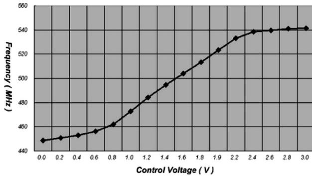
Fig. 6 Measured tuning characteristics of the VCO.
