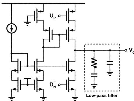
Fig. 4 Charge-pump scheme with a low-pass filter.
